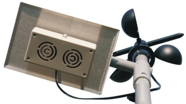
*WSI-PRO-23 Anemometer shown mounted on the AltaCom's PVC Mounting Mast and connected to the Remote Sensor Housing.*
